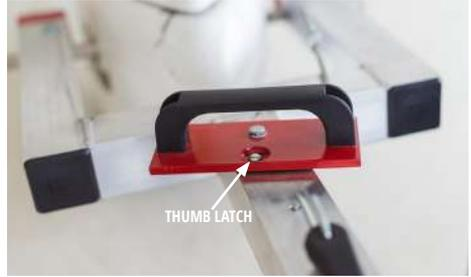
Attach to your airplane by holding both handles for alignment and then twist the attachment handle to lock it onto the lugs. Make sure the thumb latch has engaged so there is no chance it will accidentally come loose during use.
