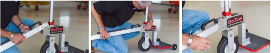
Attach tow arm to drive head with (6) included 5/16-18 x 7/8 hex bolts (**do NOT tighten until Step 8**).
