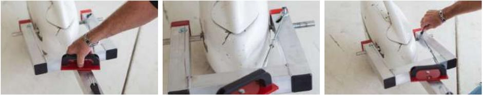
Depress the thumb latch button and move the lug tubes to the open position. If you cannot remove the GoTow from the airplane in this open position, then readjust the position of each lug tube to provide enough clearance for removal in this open position. Adjust and test in both the open and closed position until you are satisfied.
