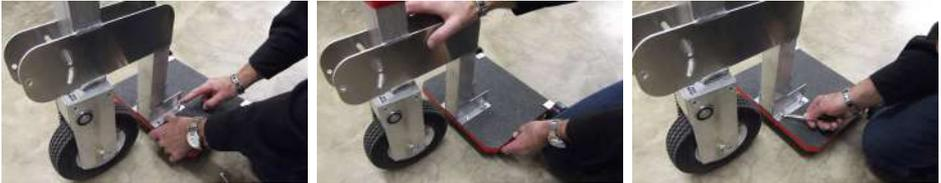
Attach the operator platform to the drive head with (4) included 5/16-18 x 7/8 hex bolts (fully tighten).
