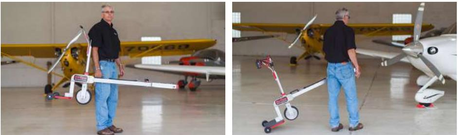
Transport the GoTow to and from your airplane by either carrying it or using the transport wheels as shown.
