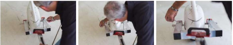
While holding the tow arm up to your nose wheel, use finger pressure to slide the lug tubes over your airplanes tow lugs on both sides. Continue adjusting the position of the lug tubes until the "fork" of the tow arm is centered on tire, then tighten both lug tube clamps.
