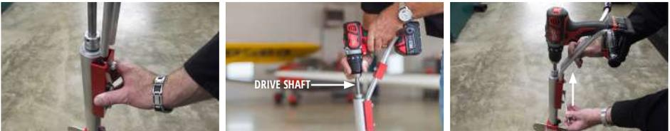
Loosen all three 5/16-18 x 7/8 hex bolts and insert handle bars to full depth. Insert drive shaft to full depth in drill chuck and tighten firmly. Finally, slide handle bars up in the channel until they are snug against the drill handle then tighten bolts firmly.
