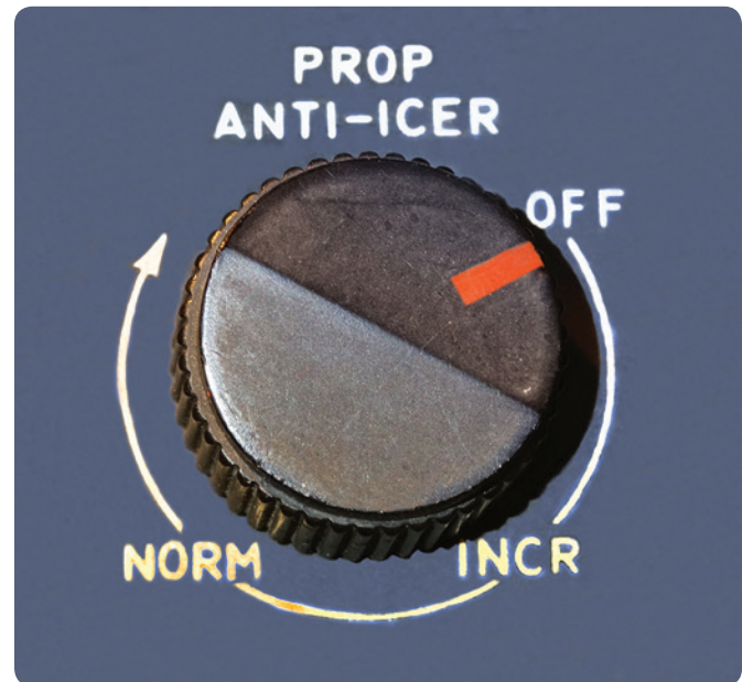
Figure 5-11. Rheostat control on anti-ice with variable flow.
