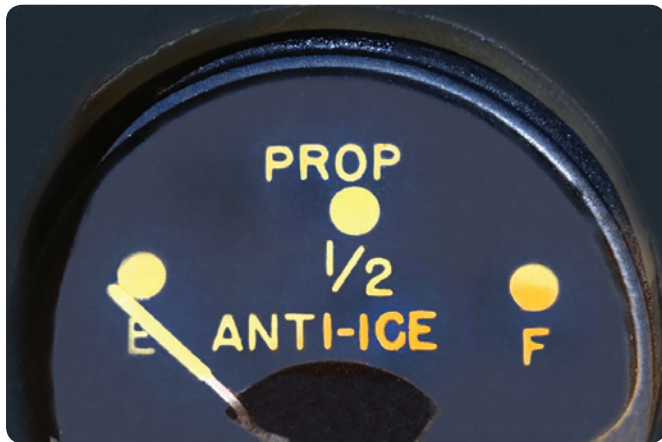
Figure 5-10. Anti-ice fluid quantity indicator.
