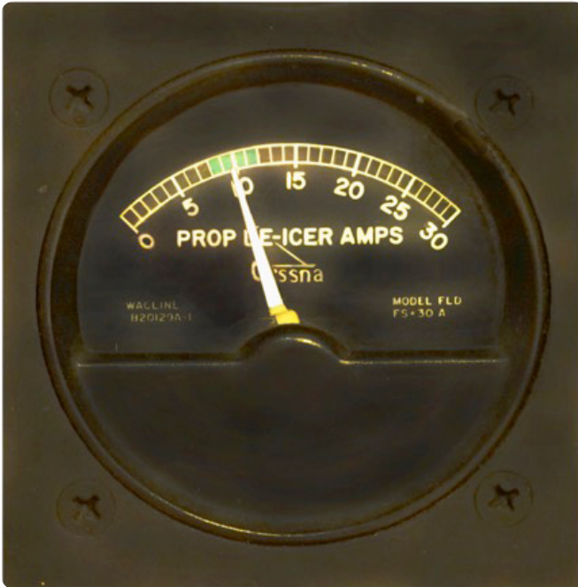
Figure 5-9. Propeller de-icer ammeter. Heating elements should draw green arc current.
