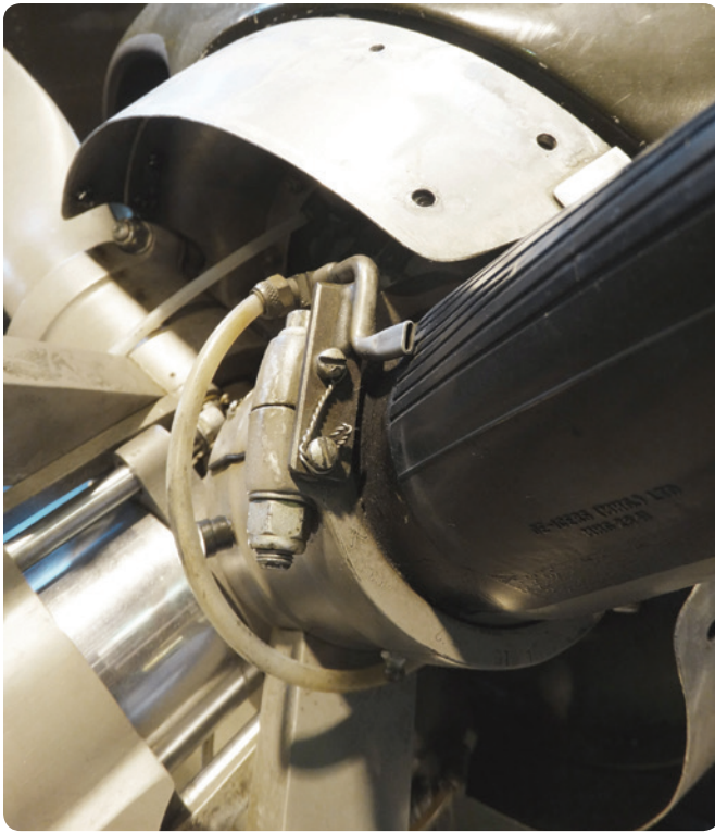
Figure 5-4. Propeller anti-ice discharge nozzle and blade boot.
