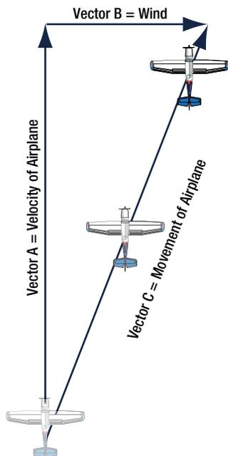
Figure 2-11. Vector analysis for airplane velocity and wind velocity.
