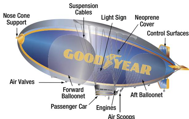
Figure 2-10. Inside view of the Goodyear airship.
