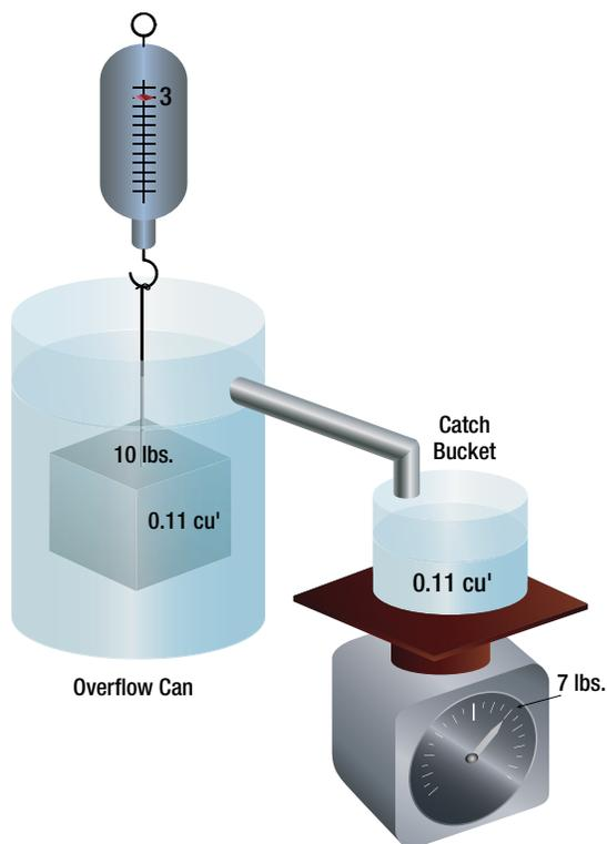
Figure 2-8. Example of buoyancy.
