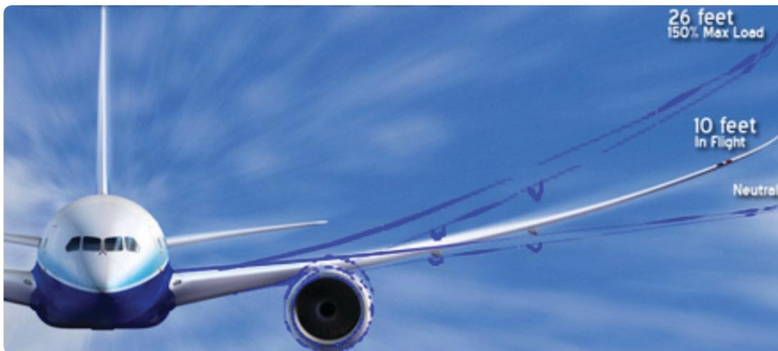
Figure 2-4. Elasticity of a modern aircraft wing aids when absorbing of stress for structural integrity and for passenger comfort.
