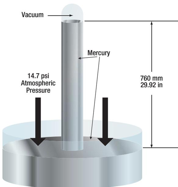
Figure 2-6. Atmospheric pressure as inches of mercury.
