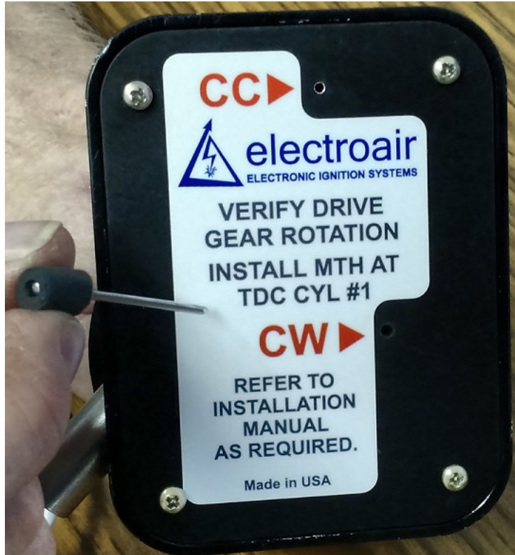
Figure 7: Installation of MTH Alignment Pin
