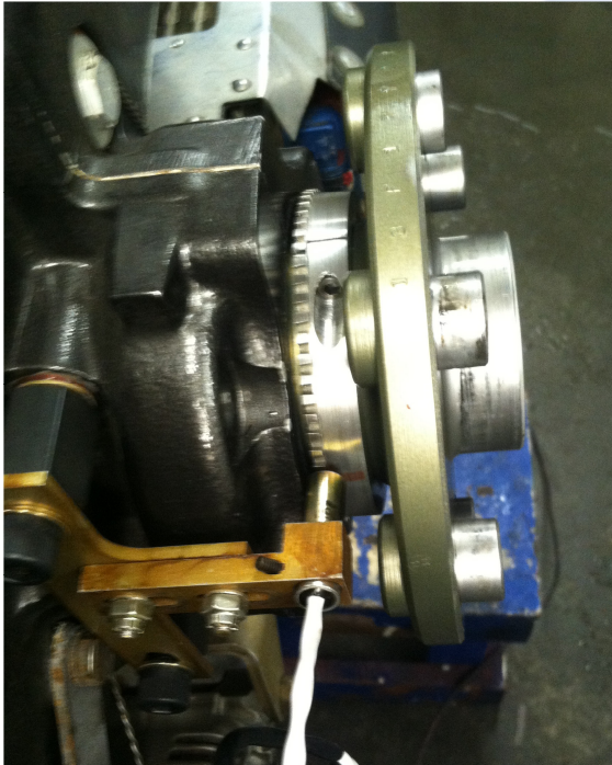
Figure 5: Picture of components that make up the Lycoming CSTW Sensor Bracket; 1. Pick-Up Bracket; 2. Pick-Up Holder; 3. Magnetic Pick-up (Magnetic Sensor); hardware is not shown for clarity.
