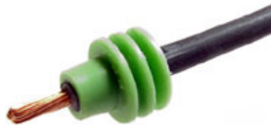
Seal loaded on stripped wire (wire stripped 5.0mm or 3/16")
