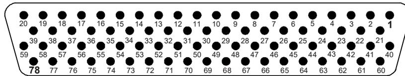
**Figure 4-11 GEA 110 J1102/P1102 Connector Looking at Unit**
