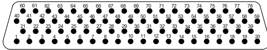
**Figure 4-2 GI 275 J2751 Connector (Looking at Connector)**
