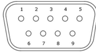
Figure 4-5 GEA 24 J241/P241 Connector (Looking at the Connector)
