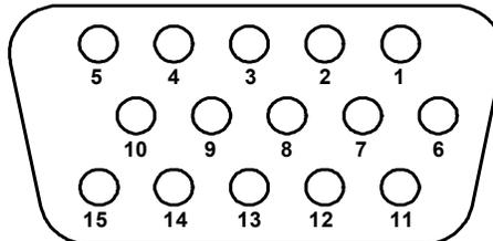
Figure 4-10 GEA 110 J1101/P1101 Connector (Looking at Connector)
