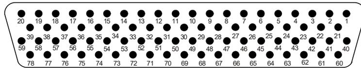
Figure 4-3 GI 275 J2752 Connector (Looking at Connector)
