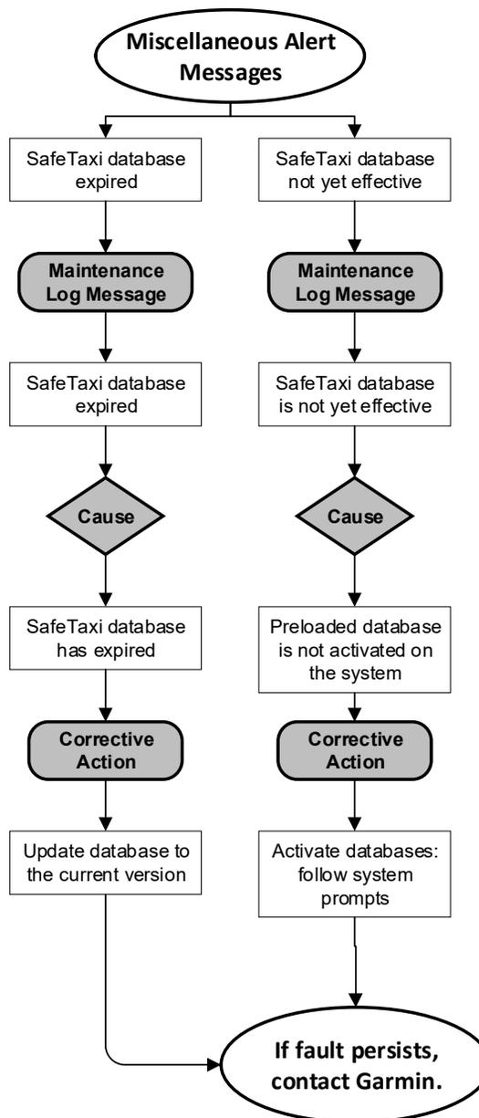
Figure 4-24 Miscellaneous GI 275 Alert Messages
