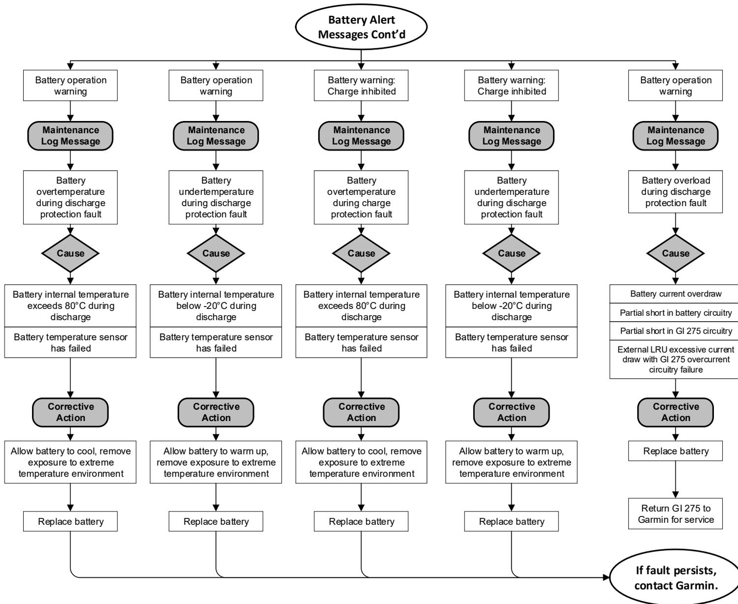
Figure 4-16 Battery Alert Message Troubleshooting Sheet 3 of 4
