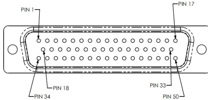
Figure 4-8 GEA 24 J244/P244 Connector (Looking at the Connector)
