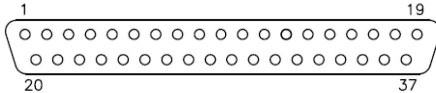
Figure 4-7 GEA 24 J243/P243 Connector (Looking at Connector)
