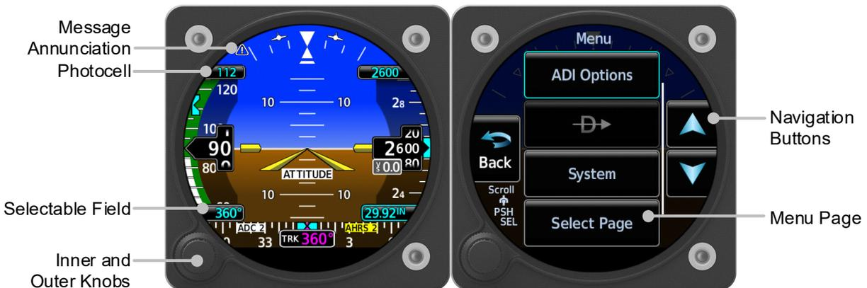
Figure 2-1 GI 275 Normal Mode
