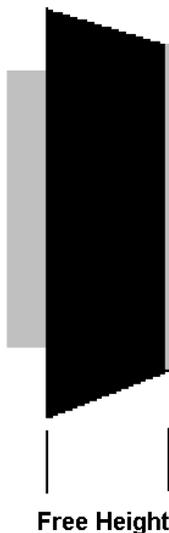
The picture to the left illustrates the free height dimension of a molded assembly. This dimension should only be measured with the molded assembly in an unrestrained (off the aircraft) condition. Table 1 at the end of this document will give the minimum heights for Barry Controls’ molded assemblies. The minimum dimension is equal to approximately 90% of the free height of a new molded assembly.
