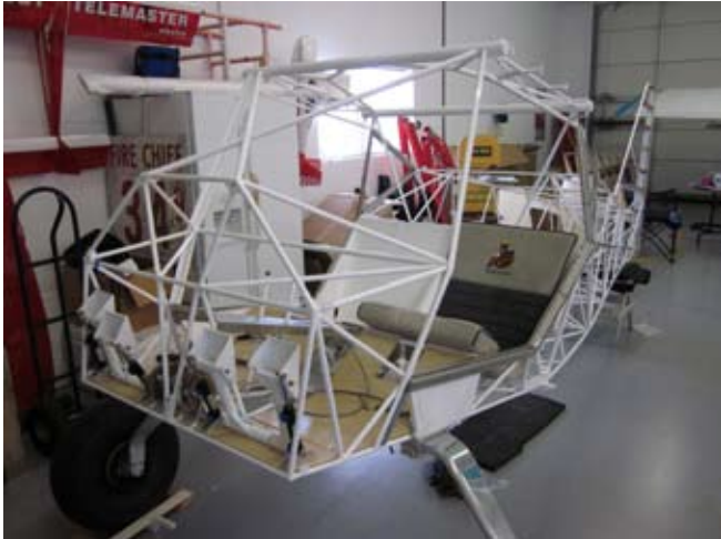
All the welding for the fuselage is done at the factory.
