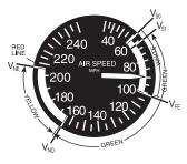
**Airspeed Indicator** Pitot-Static System
