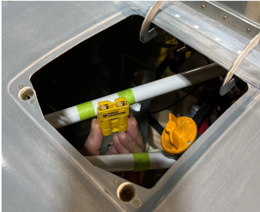
View through top cowling oil filler door opening holding SB-50 power plug in place to install.
