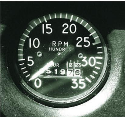
**Figure 1-30** Tachometer.
