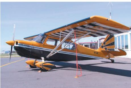
**Figure 1-16** Tail wheel landing gear.
