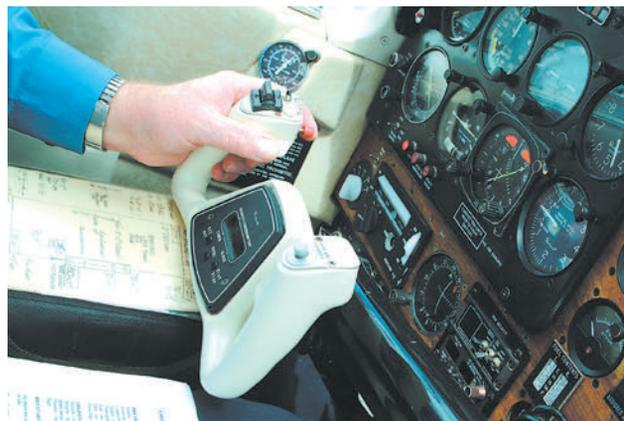
Figure 1-5 Traditional control wheel or yoke.
