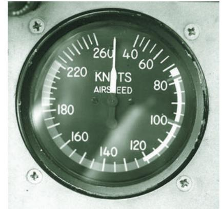
Figure 1-24 Airspeed indicator (ASI).
