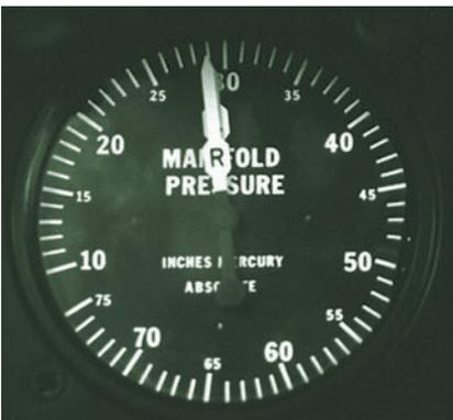
**Figure 1-31** Manifold pressure gauge.
