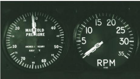
**Figure 1-14** Manifold pressure gauge and tachometer.
