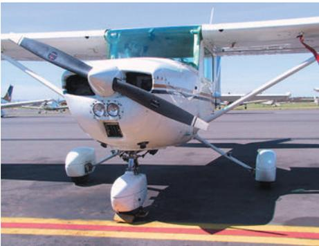
**Figure 1-15** Tricycle landing gear.
