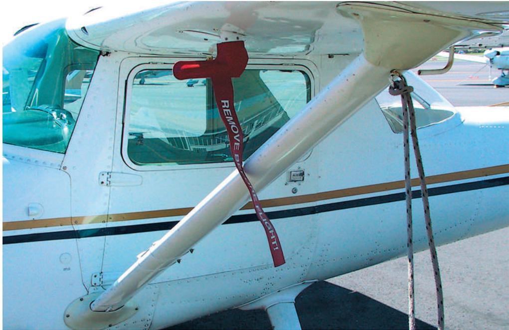
**Figure 1-35** Pitot cover and tie-down rope.
