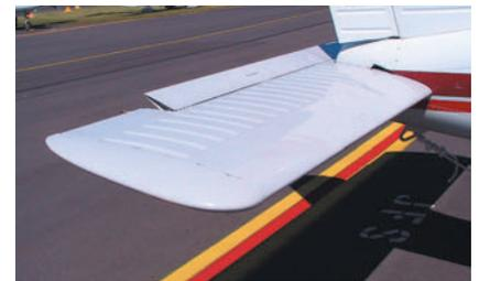
**Figure 1-11** Stabilator with tab.
