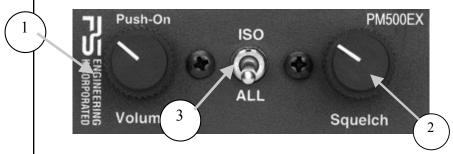
Turn the PM500EX on pressing the volume control knob (left knob). This also engages the automatic fail-safe system.
