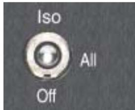
Unit power is turned on and off by the mode selector switch. In the OFF or "FAIL-SAFE" position, the pilot is connected directly to Com 1 allowing transmit and receive capability regardless of unit condition. Any time power is removed or turned OFF, the audio selector will be placed in the fail-safe mode. The switch is a 3-position mode switch that allows the pilot to tailor the intercom
