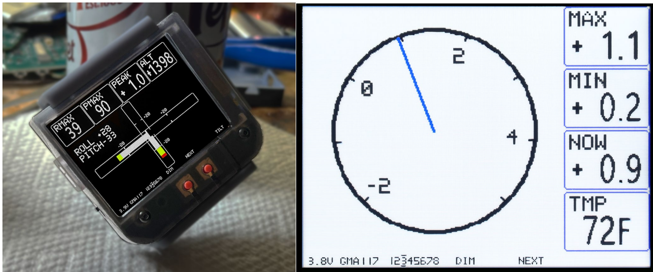
Figure 1: Automotive Roll and Pitch with black background (Selectable screen); G-Meter Basic Dial in "Paper" mode (Selectable screen)
