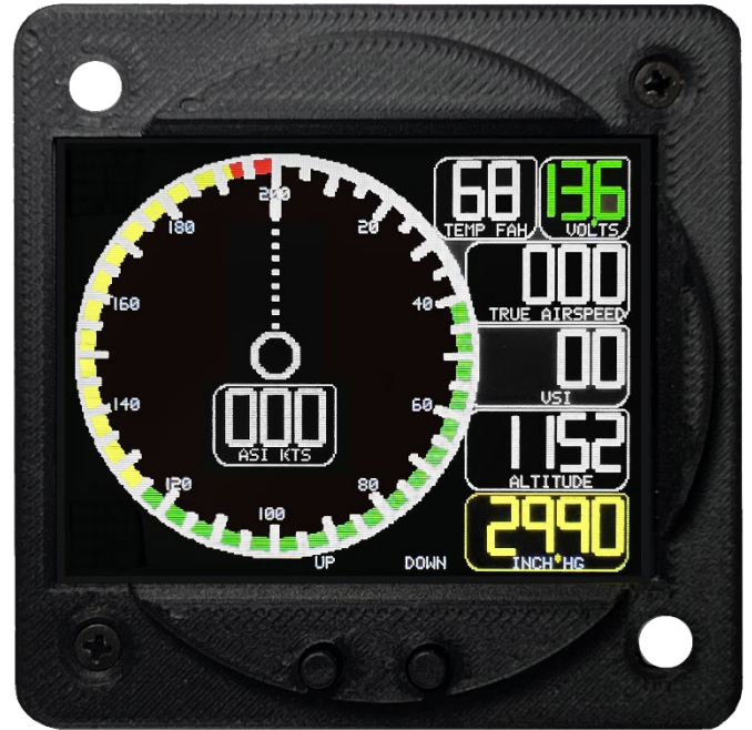
Airspeed Indicator in 2 1/4" cutout packaging showing digital / analog dial representation; OAT, system voltage; True airspeed; VSI; altitude; settable Kollsman window.
