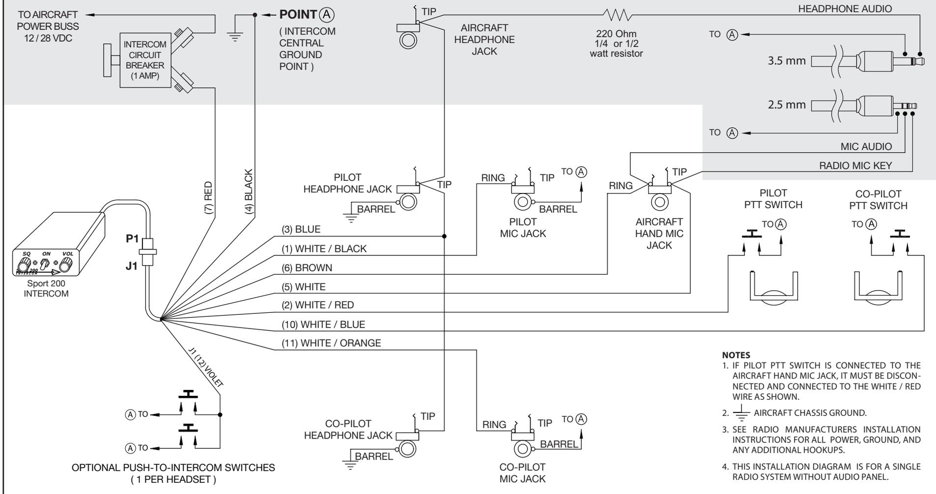
**Sport 200 – ICOM A4 Radio Installation Wiring Diagram**
