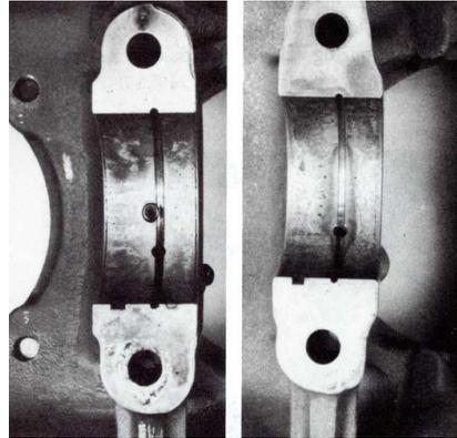
Figure 2-36. Lycoming O-320 bearing bosses. The bearing boss on the left incorporates a dowel pin to locate the bearing. A heavy wall bearing is used. The bearing boss on right does not use a dowel pin. A thin-wall high crush bearing is used. The bearing dowel functions as a locating pin. It is not designed to prevent bearing rotation. Bearing crush prevents bearing rotation.
