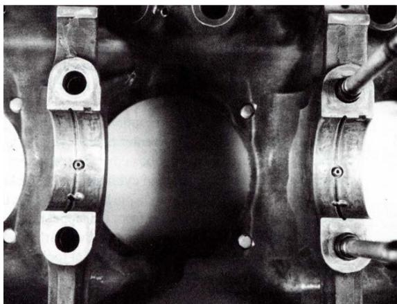
Figure 2-39. Anchored through-stud design showing dowels surrounding protruding throughstud on one side and dowel boss on the other. Dowels provide rigidity to crankcase preventing movement between the surfaces. Dowels must fit tight to prevent oil leakage out past through-studs.
