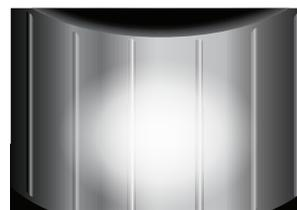
Sort contact arc indicates excessive oil clearance.
