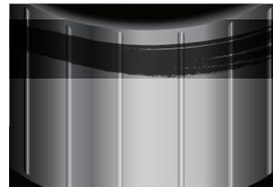
A tapered housing bore caused the distress along one edge of this pair.
