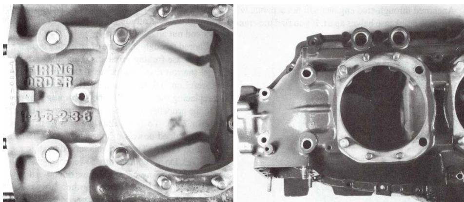
Figure 2-38. Anchored through-stud on top, body-fit through-stud on bottom.
