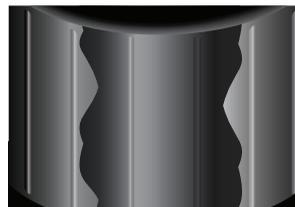
Heavy wear at thrust position of upper connecting rod bearing caused by overloading.
