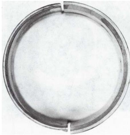
Figure 2-37. Thin wall bearing on left, heavy wall bearing on right.
