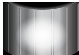
Sort contact arc indicates excessive oil clearance.
