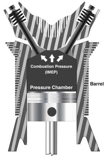
Figure 2-34. Cylinder is a cap to a pressure vessel.
