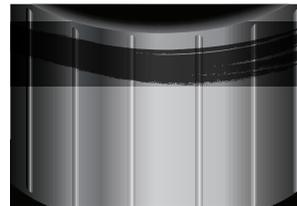
A tapered housing bore caused the distress along one edge of this pair.
