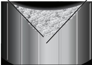
Fatigue failure of babbet material due to localized overload.
