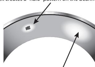
Polished and oil-stained backs are a result of a poor fit in the housing bore.
