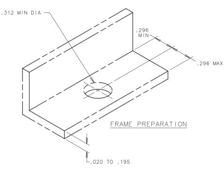
TO SELECT PROPER STUD, ADD A CONSTANT OF .030 IN. FROM THE TOTAL OF OUTER PANEL THICKNESS, FRAME THICKNESS AND SPACE BETWEEN THE TWO. NOTE: THE SPACE BETWEEN THE OUTER PANEL AND FRAME WILL ALWAYS BE AT LEAST .025 IN. BECAUSE OF THE THICKNESS OF THE RECEPTACLE LEG, AND MUST ALWAYS BE INCLUDED IN THE TOTAL.
