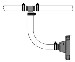
For aircraft with ¼ inch static lines, two adapters are provided which can convert from ¼ inch inside diameter hoses to the 5 mm hose in the install kit.
