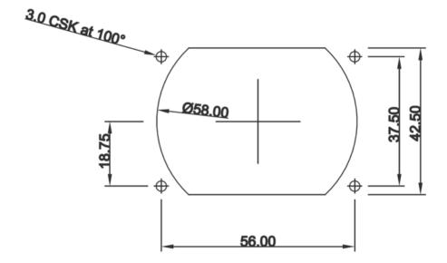
Note: The following diagram is intended to be to scale, however variations in the printing process mean that you MUST check all dimensions before using it as a template.
