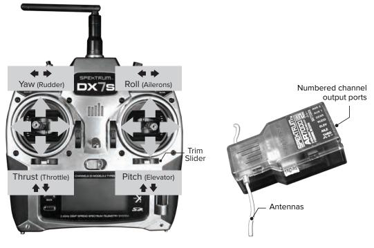
Figure 1-1. RC transmitter, mode 2 configuration.
