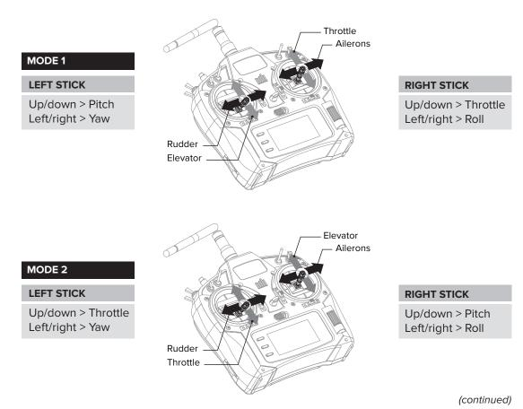
Figure 1-3. RC transmitter modes and channel assignments.
