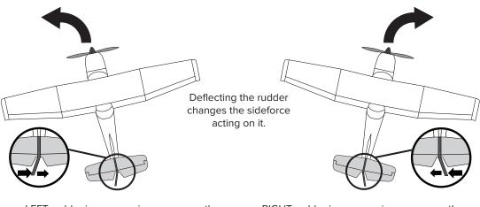
LEFT rudder increases air pressure on the left side of the fin; aircraft yaws left.
