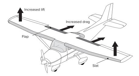
Figure 1-15. The location and function of flaps.
