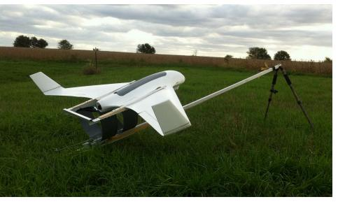
Figure 2-4. A catapult may be used in the absence of a suitable runway for takeoff.
