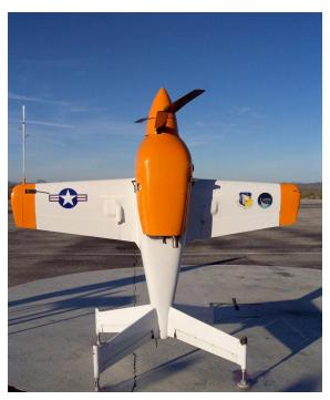
Figure 2-8. Takeoff and landing position of tail sitter unmanned aircraft.
