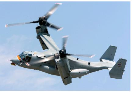
Figure 2-6. Osprey tilt rotor aircraft transitioning to forward flight.
