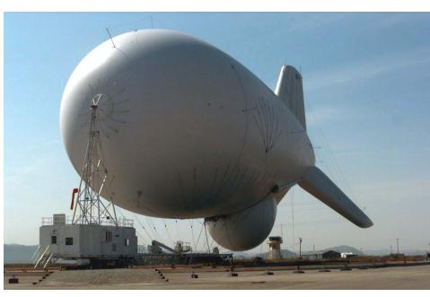
Figure 2-10. An aerostat type airship with tethering tower.
