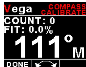
Fly a number of banked 180 or 360 degree turns at different bank angles - i.e. shallow, medium and steep turns. Try to add many different pitch attitudes in various orientations relative to the field direction. It does not matter in what order you fly the maneuvers. A typical, good calibration tends to take 5-10 minutes of flight.
