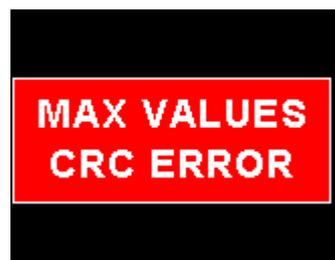
Max Values CRC error. Load default settings to restore to factory defaults. If the error message still persists then it could possibly be a non-volatile memory failure in which case the instrument will then have to be returned to the factory.
