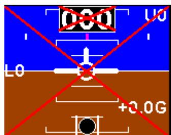
The display will have a red cross over the indicators to signal a SP-X sensor communication or sensor failure. Check the communication link between the AHRS-1 / MAG-1 and the SP-X sensors and that the SP-X sensors themselves are functional.
