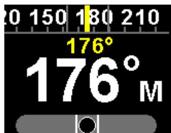
The F1 key pressed at a heading of 176 degrees. Currently the heading equals the course to steer as shown below the heading tape. No course steering indicators are shown.
