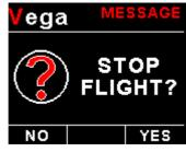
Press the F1/Up button during the normal display mode to manually start/stop a flight. This key is only active if the ASI-4 is setup to select the manual flight option under the "TIMERS" setup menu.
