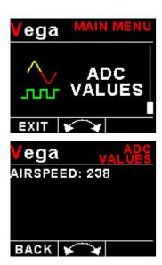
This menu displays the ADC value that have been read from the airspeed pressure sensor.
