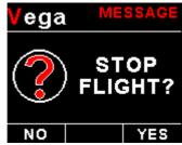
Press the F1/Up button during the normal display mode to manually start/stop a flight. This key is only active if the ASV-1 is setup to select the manual flight option under the "TIMERS" setup menu.
