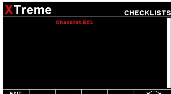
Copy the created file (.ECL extension) to the checklst directory on the SD card when you are complete. The checklist file can be loaded by pressing the rotary control and selecting "CHECKLISTS". A window containing all the files with the .ECL extension will be shown. Select the checklist you require. The number of checklists that can be stored and displayed depends on the size of the SD card.
