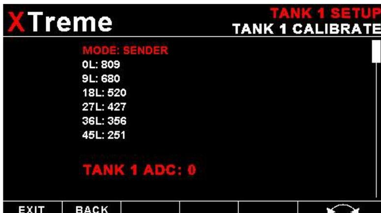
Select “SENDER” for the “MODE” menu item. Once you have installed a fuel level sender into your tank, make sure the float can travel all the way from empty to full position without hindrance of any kind. The calibration procedure should be carried out with your aircraft in flight attitude. This means you need to lift the tail if you have a tail-dragger or lift the nose wheel if you have a weightshift trike.
