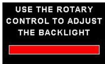
Select this menu option to adjust the backlight brightness level. This may be desirable during low light flying conditions. Use the rotary control to adjust the brightness level.
