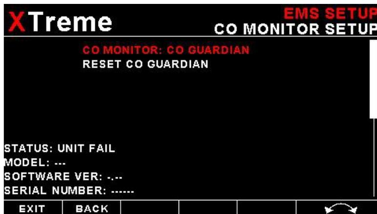
The CO Monitor Carbon Monoxide menu option allows the pilot to enable the CO Guardians Carbon Monoxide detector. The XTreme-EMS will display the carbon monoxide value on the EMS display as well as enable the carbon monoxide warning alarm. Please see the relevant CO Guardian detector manuals for more information.
