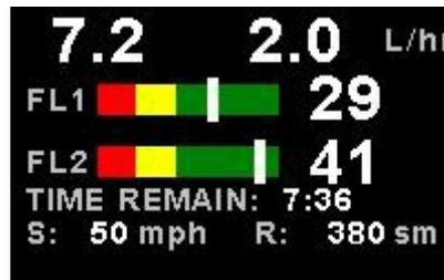
**3.1.4.3 Single fuel flow and dual fuel level senders (dual tank)**
