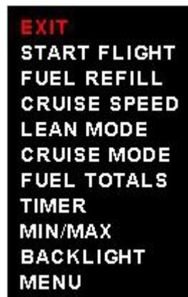
Press the rotary control when the EMS screen is displayed to access the EMS quick select menu.
