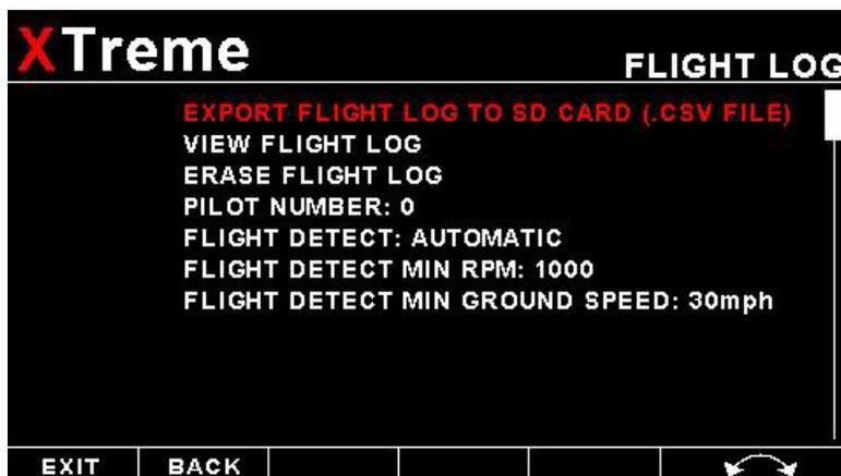
**NOTE:** The Flight log is stored in RAM until a valid flight has been completed. If the power is turned off to the XTreme-EMS before the flight has ended then the flight information will be lost.
