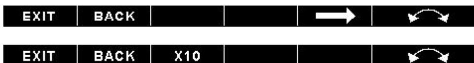
Use the menu sub-bar for quick menu navigation. Select the soft key directly under the text to activate the softkey function. Some soft keys have a x1, x10, x100, x1000 assigned to them. This allows for faster incrementing and decrementing of the menu settings.
