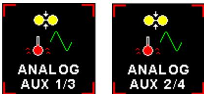
The analog AUX 1/3,2/4 channel on the RDAC are general purpose channels that can be used for pressure, temperature or current. The AUX 3 and 4 pertains to the RDAC-XF / MAP and AUX 1 and 3 to all the other RDACs.
