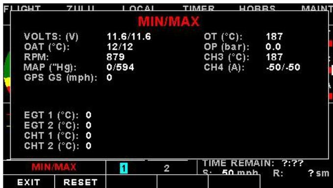
Select this menu option to display the maximum and minimum captured values. Press the “RESET” soft key to reset the min/max values to the current values.
