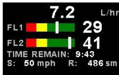
**3.1.4.4 Single/Differential/Summed fuel flow, single fuel level sender, single calculated tank**
