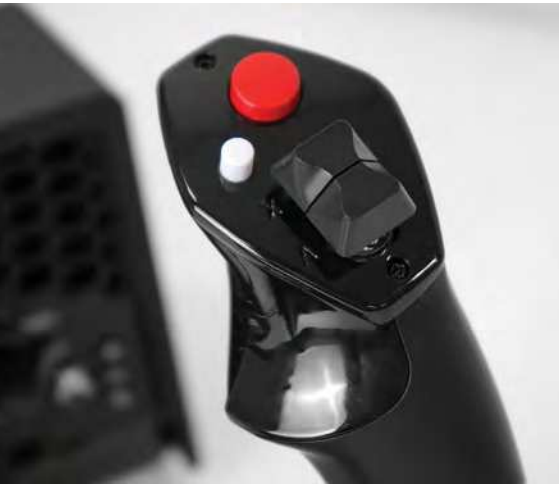
Above: Twin rocker switches and two push-buttons can be configured for functions such as aileron and rudder trim.
