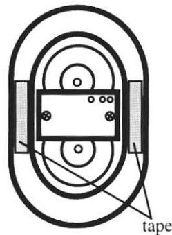
When audio system and anr system work properly, remove earseals and withdraw module only enough to allow removal of exposed backing paper from tape. If module is removed from earcup, check to see that wiring, etc., remains tucked out of the way. Press module firmly into earcup.
