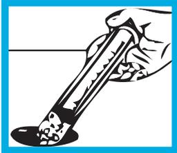
1. Remove cap from can and insert dispenser snugly with plunger all the way down.
