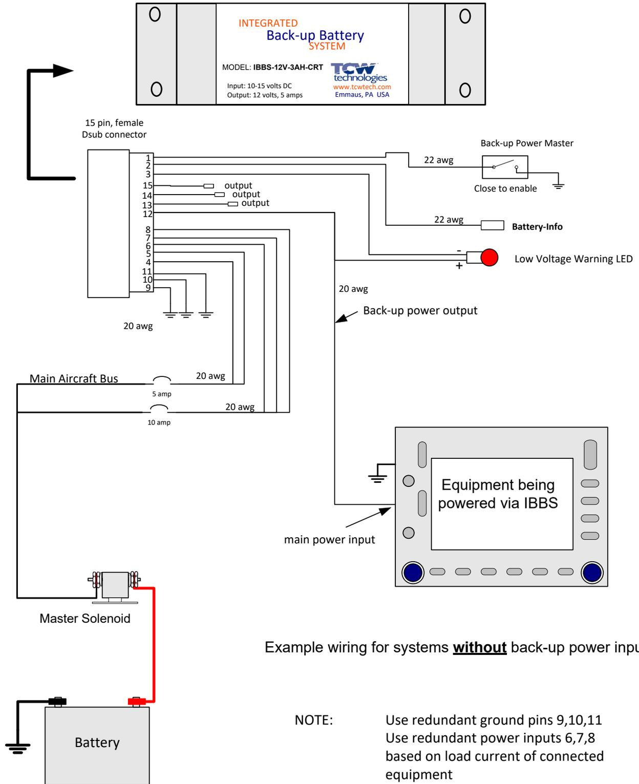
Example wiring for systems without back-up power inputs
