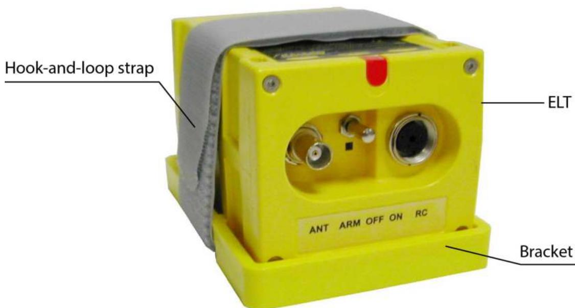
Figure 6: INTEGRA ELT with Mounting Bracket P/N S1840502-02
