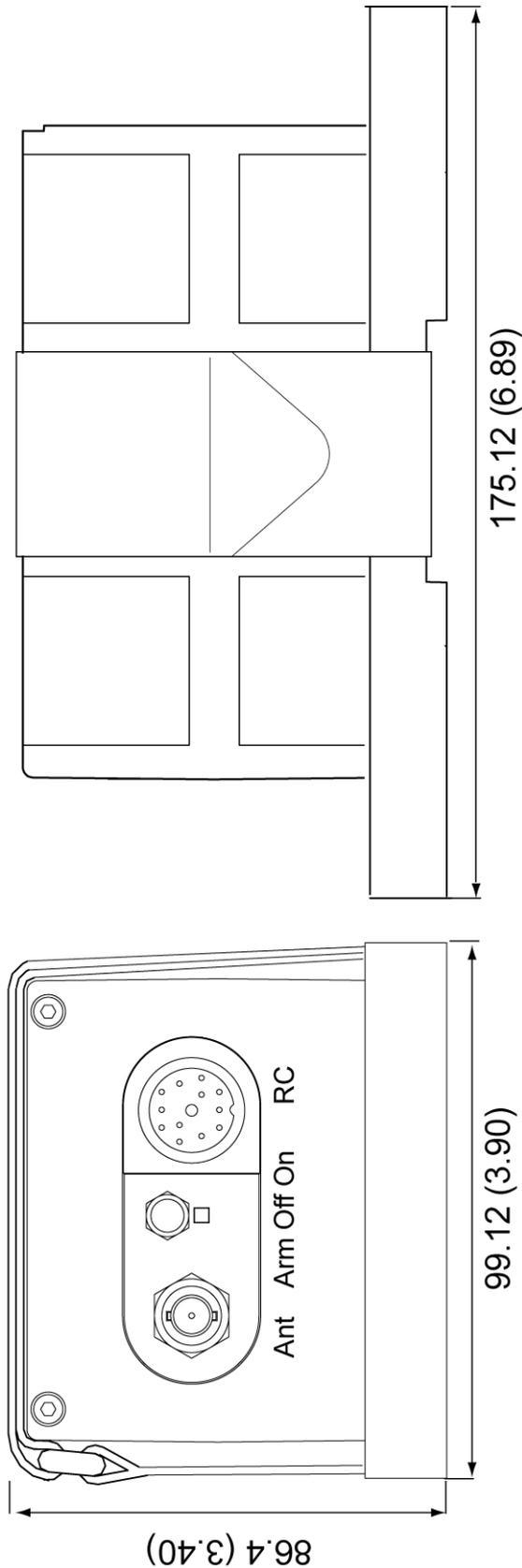
**3. Outline dimensions and weight with Bracket Universal for INTEGRA ARINC e-NAV for ELT (AF) P/N S1850551-02**
