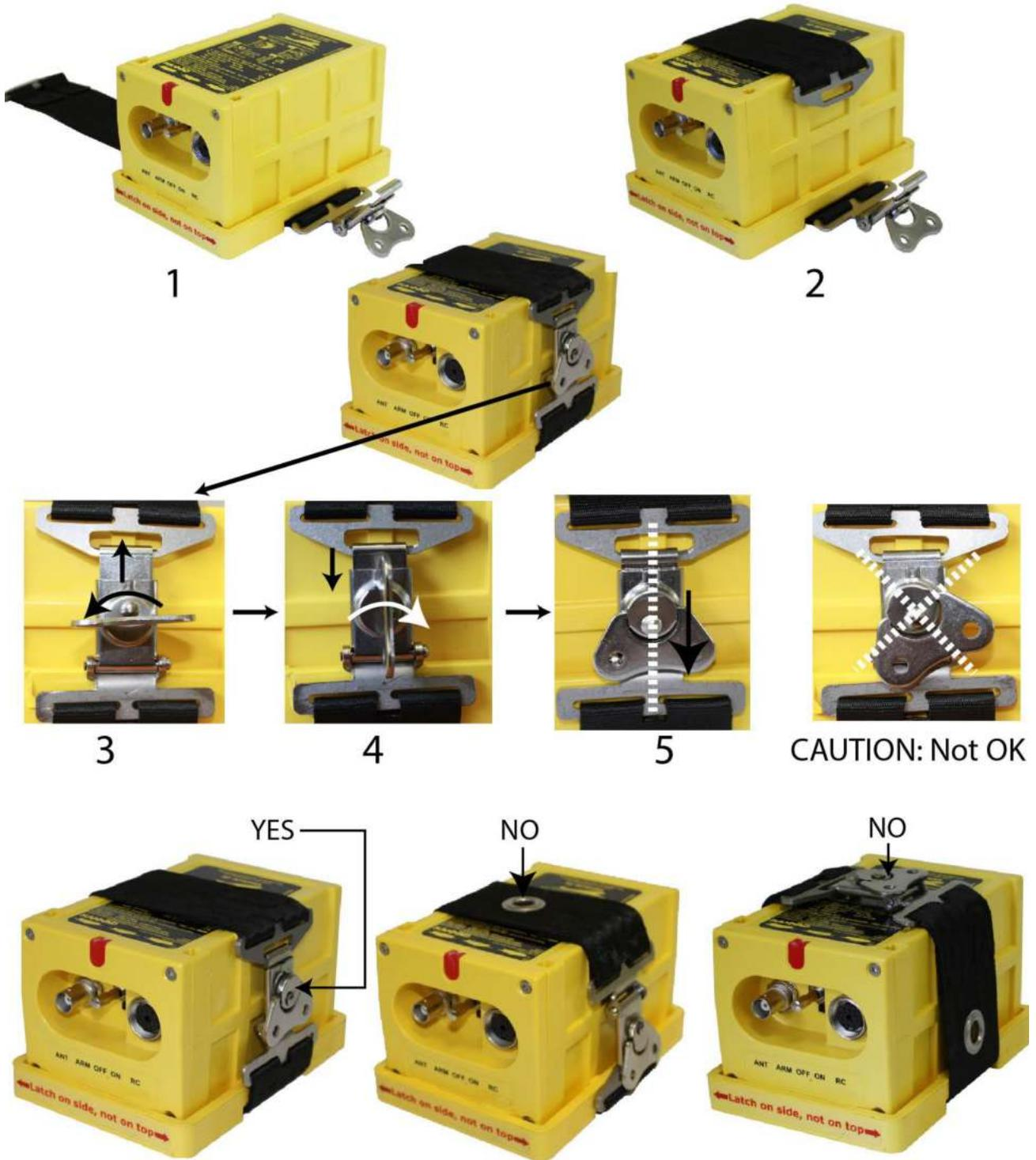
CAUTION: Never install the strap with the latch or grommet on top of the ELT
