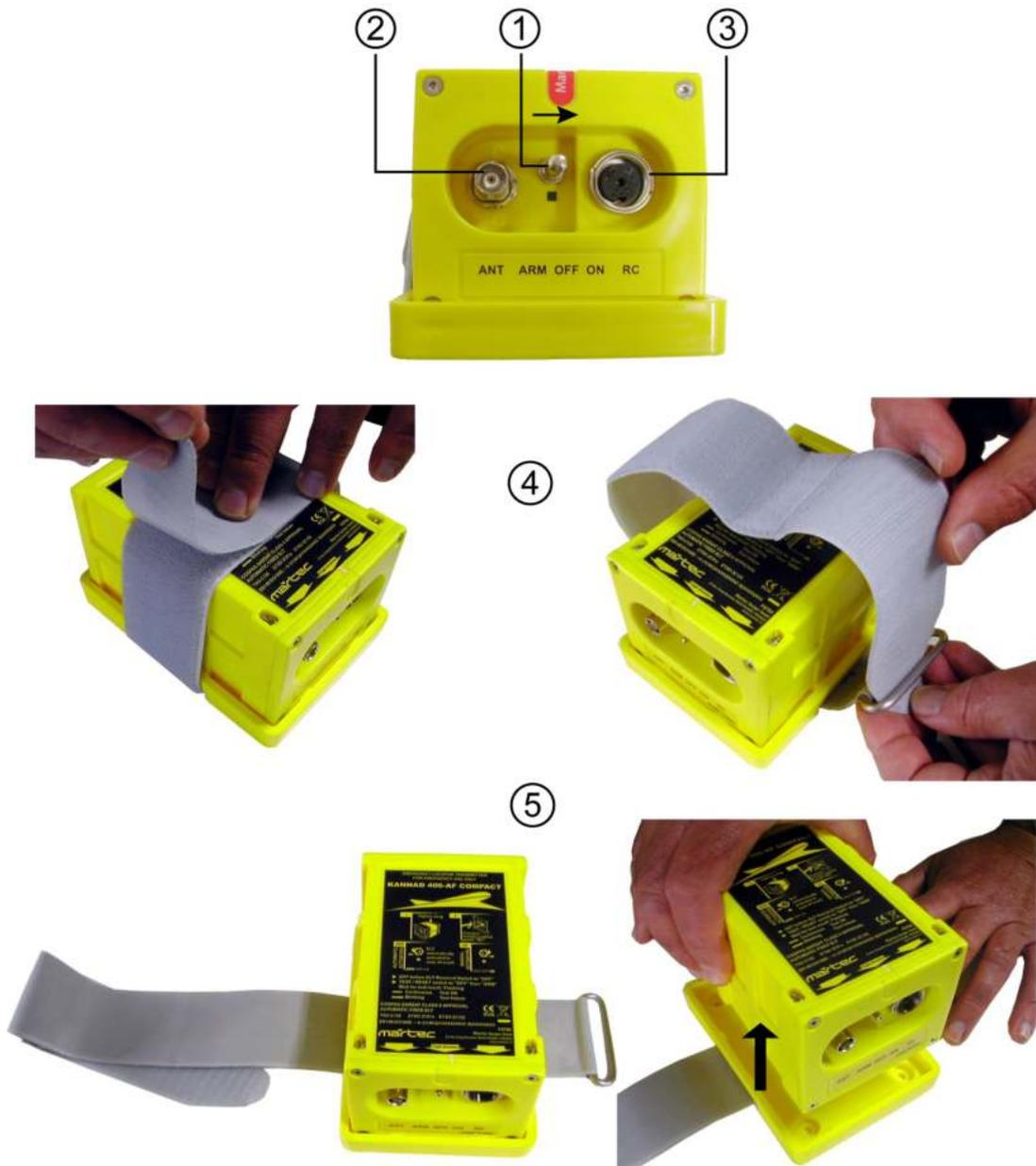
(2) Removal of the ELT from a draw latch mounting bracket
