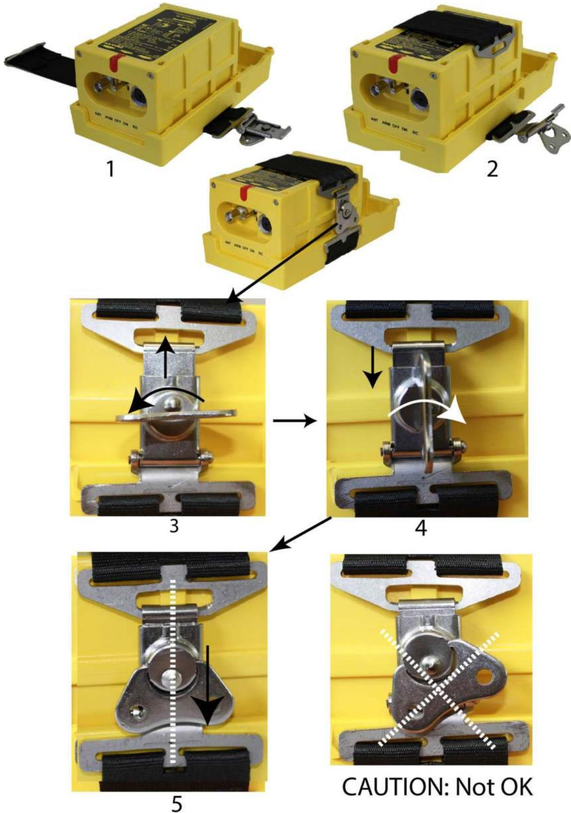
*(3) ELT installation with draw latch mounting bracket P/N S1850551-04*
