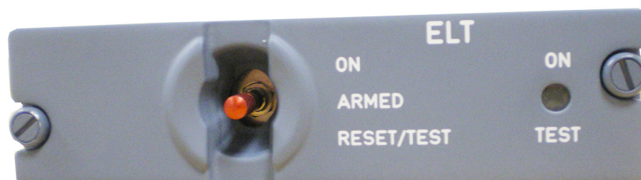
Figure 14: RC800 / 810 Remote Control Panels
