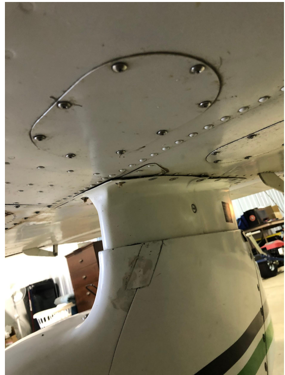
Example of installation on a Piper Warrior with a replacement access panel
