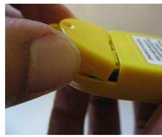
**6. Replace cover, as shown. Cover will snap into place. Replace screw.**
