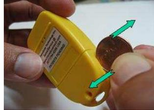
**2. Use coin to remove battery cover. Turn coin *clockwise*. Battery cover will pop off.**
