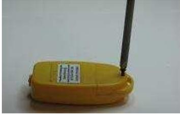
**1. Turn Pocket CO off. Remove screw, and put aside (don't lose it!).**
