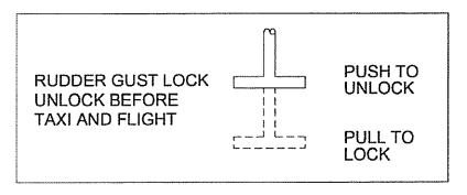
On either side of the nose gear fairing, above the towbar attachment points:
