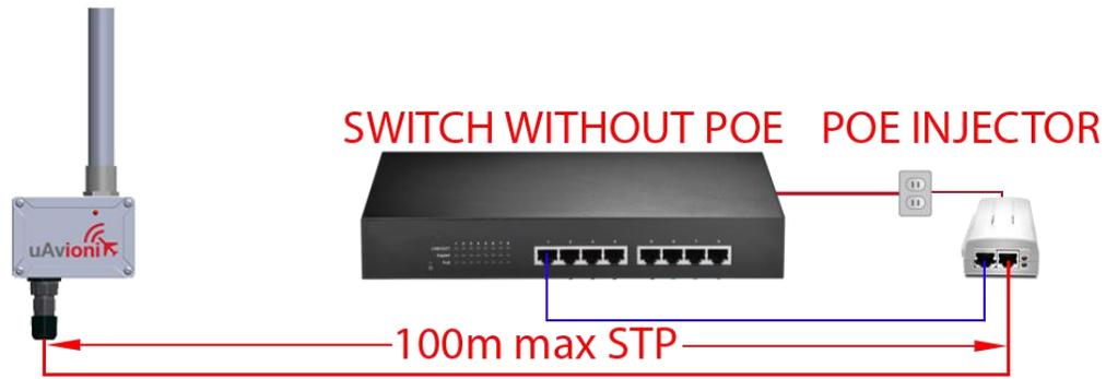
PingStation install with POE injector
