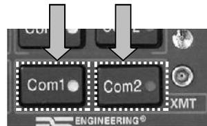
Select either of the com XMT buttons to exit the split mode. It is not possible to have the pilot on Com 2 and copilot on COM 1 in split mode.
