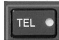
The TEL mode serves as a full duplex interface and distribution for telephone systems such as portable cellular phones with earpiece jacks or Bluetooth connectivity. Pressing the button connects the telephone to the users as follows:
