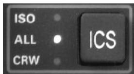
**ISO:** The pilot is isolated from the intercom and is connected only to the aircraft radio system. He hears the radios (and sidetone during radio transmissions). The copilot and passengers will hear the music sources as configured by the audio panel configuration Function keys. See page 11—Smart
