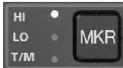
Pressing the MKR button for one second will cause the marker audio to mute. The next beacon received will re-activate the audio.
