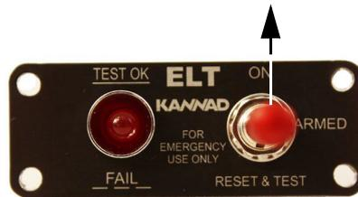
Pull and lift upwards
