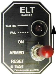
Pull and lift upwards
