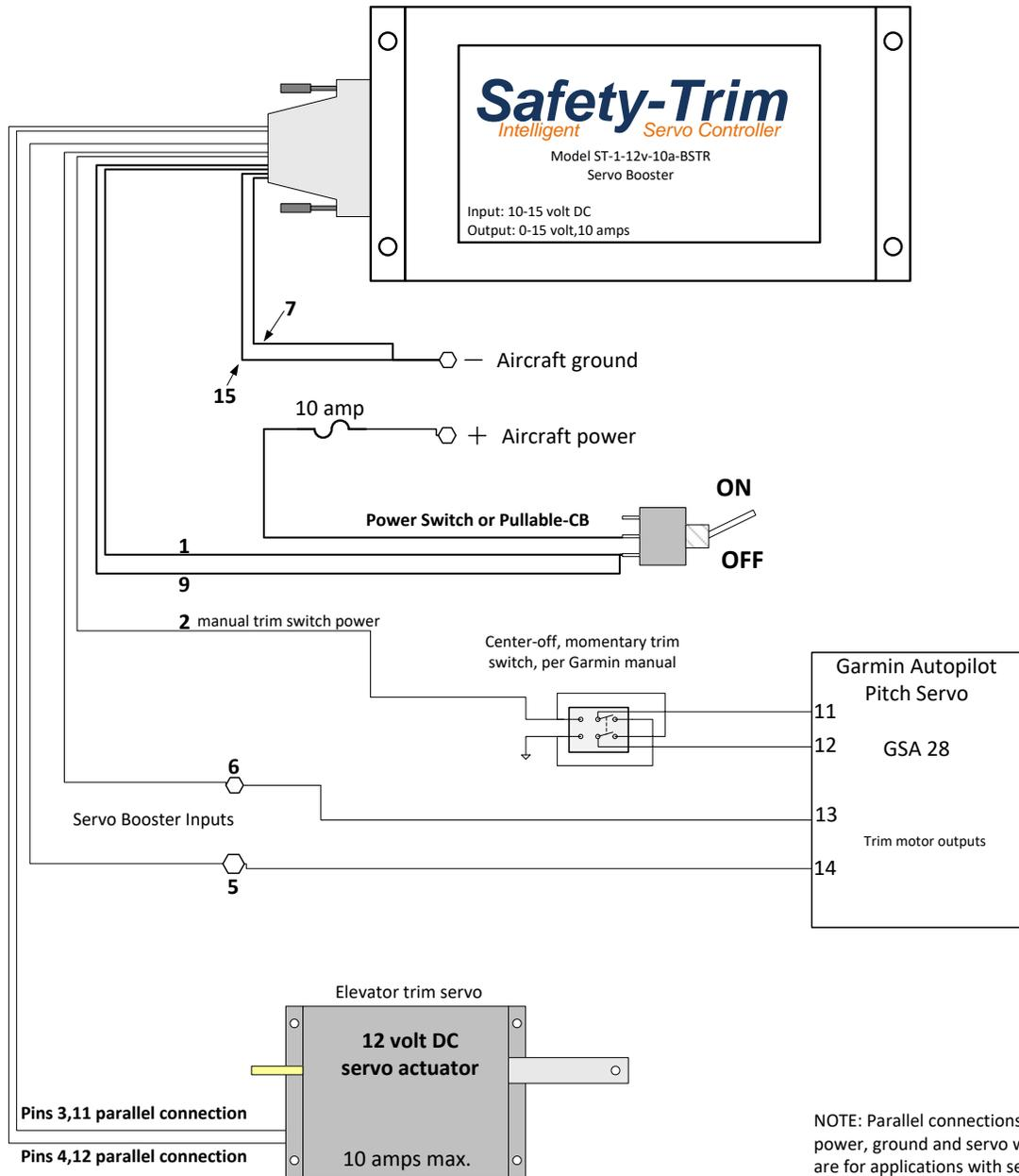
NOTE: Parallel connections of power, ground and servo wires are for applications with servos rated at more than 5 amps
