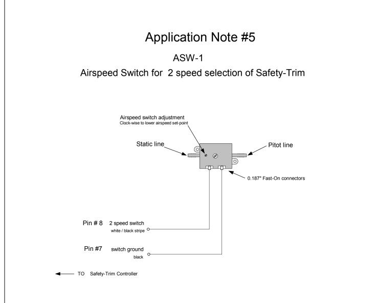
Note: Pin #7 is a common switch ground for all trim switches and the airspeed switch. An airframe ground may be used as an alternative
