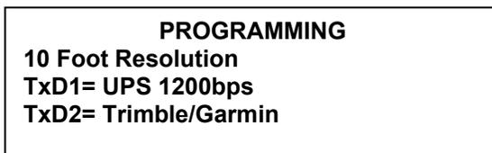
**Step 7:** Confirm the port programming by pressing the **READ SET-UP DATA** pushbutton. It should display the settings applied in the previous steps. In the case of our example the display would appear as below.
