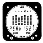
To display the Temperature Below Peak EGT (example: "PEAK -25), push the Mode Switch to the left.
