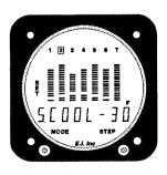
Shock Cooling Rate (S.COOL) is displayed in degrees F per minute for the indicated channel inside the lit box.
