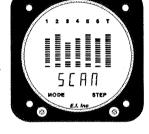
When operating in the Scan Mode only, program the Scan Rate by pushing and holding the Mode
