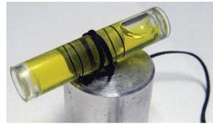
This extremely simple and sensitive tool uses the plum-bob and bevel principle to balance props both vertically and horizontally. It can be carried in a small tool box for easy use in the field and balances props accurately for smooth operation. The precision machined hub works with any prop designed with standard 1" center
