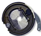
These 4.5" brakes have a long actuating arm, 5/8" mounting hole, and bonded lining. Available in anchor style w/ built-in anchor & 2 cable mounting ears, or round style which features a round aluminum backing plate. Platform required w/ 5" Azusalite.
