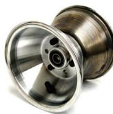
**6" SPUN ALUMINUM NOSE WHEEL** - The 6" Spun Aluminum nose wheel with 5/8 bearings. Comes centered when using the MX o-ring standard wheel hub but can also be purchased with the MX offset hub (no o-ring with offset hub. Requires the use of a tube. Comes complete with nuts, bolts, washers, valve stem, o-rings if required and the MX hub. May also be used as main wheels.
