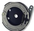
These 5" brakes are used on Azusa #1175 wheels only. Features a round aluminum backing plate and actuating arm which allows for 8 positions.
