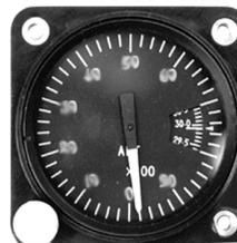
The mini altimeter is a remarkable instrument. Through the use of an accurate single pointer design, the 0-5,000 and 0-10,000 altimeters are able to squeeze precision and reliability into a 2-1/4" instrument which is less than 2" deep. All altimeters are designed with Kollsman windows, glass faces, precision jewelled movements and a rugged combination metal and plastic case. Static porting is standard. 0-5000 ft. Altimeter, Millibar
