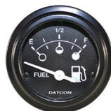
This Datcon fuel gauge and senders are designed for use with 12 volt electrical systems in automotive, marine and homebuilt aircraft applications. The gauges have a round 2" diameter case with chrome bezel. Mounting brackets and instructions are furnished. 240-33 Ohms. Gauge No. 100177 with steel case ..... P/N 100177 ..... **\$58.75**
