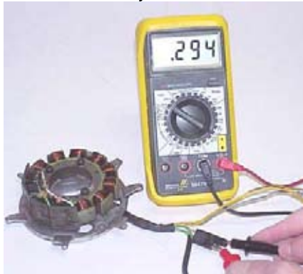
Figure #3 – Shows the test for a new style stator output leads across the white and green leads. The chart shows an expected value of 280 to 330 ohms. Meter shows 294 ohms. The part checks good.
