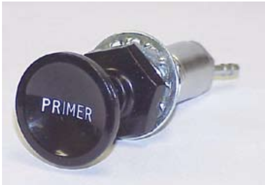
Figure #8 – A Plunger Primer is a great addition to aid in cold starting but in no way can be used as a diagnostic tool.
