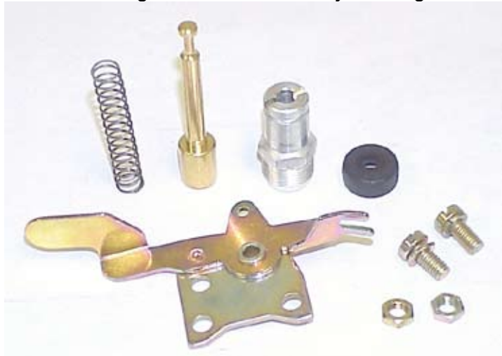
Figure #4 – Lever style chokes are the simplest type of actuator that is pretty much self contained. Being able to reach this safely in flight is essential to diagnose problems. Order Part #7658 for this kit.
