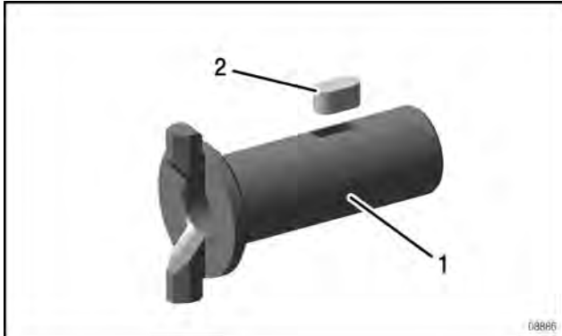
1. Oil pump shaft
