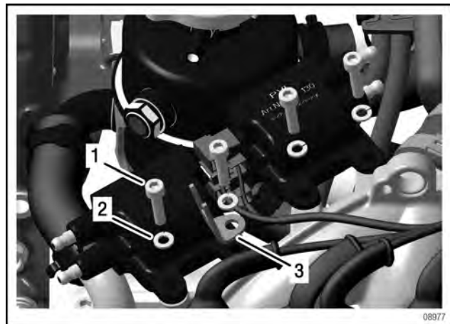
1. M5x16 Allen screw 2. 5.3 washer 3. Plug holder
