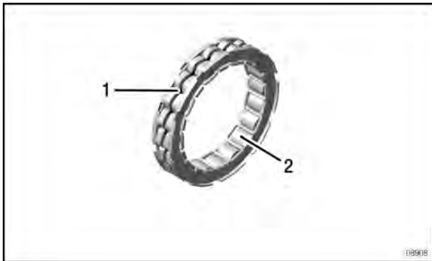
1. Helical spring 2. Spear body
