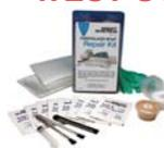
Useful for a wide variety of fiberglass repairs, including repair of cracks, scrapes, loose hardware, gelcoat blisters, delaminated cored panels, holes, keel damage, and more. Kit contains eight pre-measured packets of 105 Epoxy Resin and 205 Fast Hardener (19.2g mixed), adhesive filler, fairing filler, mixing cups, fiberglass fabric, reusable mixing stick/applicator, syringe, two coating brushes, three pairs disposable neoprene gloves and complete handling and repair instructions. Kit 105-k.
