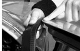
The "Spring-Steel" reinforcement channel has "Gripper" teeth to hold firmly in place. And when your door is closed the seal is pinched between the airframe. You can not pull the seal out when the door is closed...however applying adhesive into the channel is recommended. Length: 9ft. P/N 05-02203 .....\$159.75
