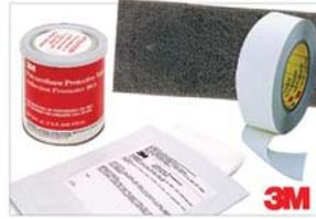
Designed for experimental aircraft that have been identified as needing gap seals to improve control response and effectiveness. Features transparent, UV stable film with a long aging, acrylic adhesive. Remains flexible down to -40 deg. F. Easy to install with the use of simple hands tools. Kit includes 3M 8674 Film (PN 09-01643), 86A Adhesion Promoter to ensure maximum adhesion, Scotchbrite pad (PN 09-01753) and 3M Application Solution (PN 06-00604)
